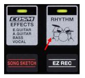
The BR-800 provides a dedicated rhythm generator that is separate from the audio tracks 1-8. You can use this rhythm as a guide during recording, or create an original rhythm backing by arranging various internal rhythms to match the structure of your song. Let's create a rhythm arrangement consisting of various patterns.
