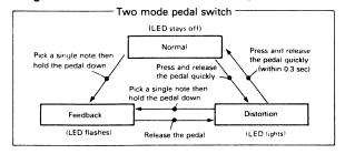
The DF-2 adopts the unique two mode pedal switch system that allows changing the mode like Normal  $\longleftrightarrow$  Distortion  $\longleftrightarrow$  Feedback by pressing the pedal. Please study the figure shown left for proper operation
