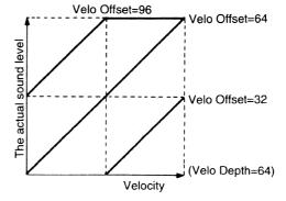
The actual volume that results from how hard you play a key will depend on the Velocity Sens Depth and Velocity Sens Offset as shown in the following diagrams.
