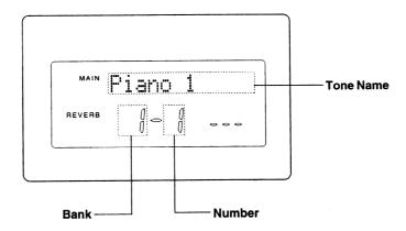
Try switching a few Tones and playing them using the connected MIDI keyboard. Or, if you aren't hooked up to a keyboard, just press the  $(\bullet)$  button to hear the currently selected patch.
