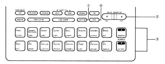
1 Press the UTILITY button as many times as necessary to select the screen shown below.
