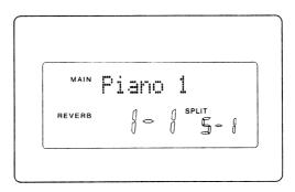
The keyboard is divided into two sections, upper and lower, and you can specify the key that will be the boundary between them (the "Split Point"). A different Tone can be assigned to the upper and lower keyboards.
