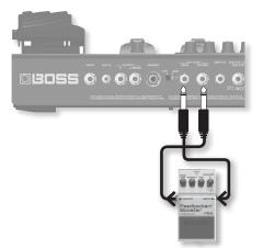
The sound that is input to SEND/RETURN within the effect chain will be output to the SEND jack. The sound that is input via the RETURN jack will be input to SEND/RETURN within the effect chain.
