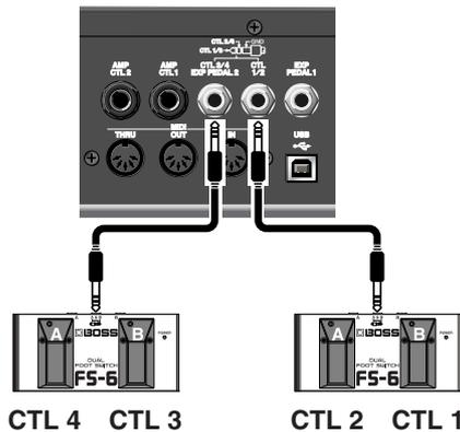
\* The following shows the correspondence between the foot switch and CTL function when two foot switches are connected using a special connection cable (Roland PCS-31; sold separately).
