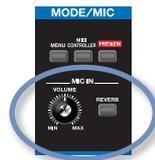
Hold down SHIFT and press the MIC IN area’s REVERB button to display the MIC IN SETTINGS screen.
