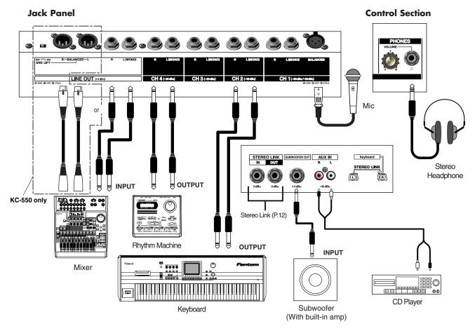
Here is an example of a setup that makes full use of the KC-550/KC-350's mixer and monitor functions.
