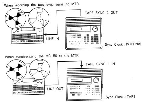
To synchronize the MC-50 to an MTR, set the sync clock (\$\sigma\$P.62) of the MC - 50 to "TAPE". Playback will begin when a tape sync signal is received from the TAPE SYNC II jack.
