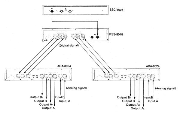
\* DIGITAL OUT channels 1-4 on the RSS-8048 correspond with channels 1-4 on the SSC-8004.
