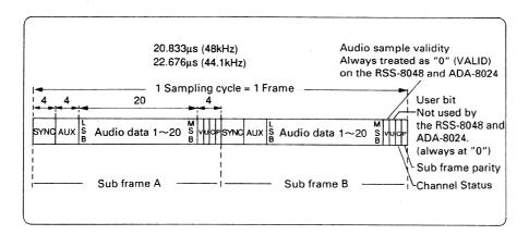
Channel Status accumulates 24 bytes as a result of 192 frames (192 sampling cycles), and is concluded as one block. (192 frames is referred to as one block.)
