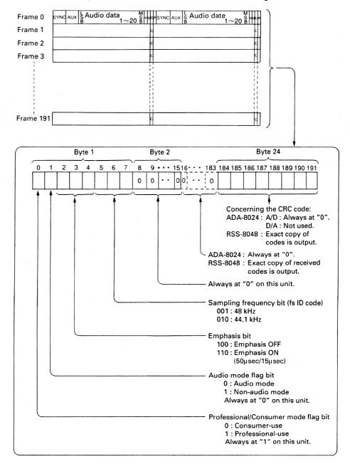
IMPORTANT: In this system the last byte (24) of the Channel Status (CRC code) is not generated. Should you ever need to connect external equipment that "looks" for the CRC code, you must first turn off that function on that unit.
