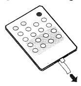
The remote control unit contains a lithium battery. An insulation sheet is inserted to keep the battery from discharging. You must remove this insulation sheet before using the remote control. Grasp the tab and pull the sheet out.
