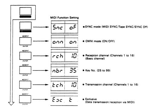
When you would like to change the setting of a particular MIDI function, first get the required MIDI function in the display, then change it while holding the Shift Key down.
