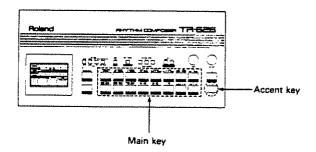
Each of the Main Keys 1 to 14 have been allocated 2 drum voices. These two voices' names are written above each Main Key on the front panel.
