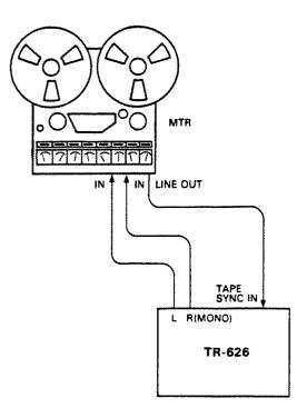
Rewind the tape onto which the synchronized signal was recorded. Find the part of the tape where a pilot tone is heard before the modulated tone begins. This is the place from which to begin.
