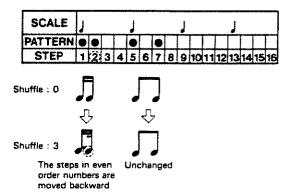
Step 1 While pressing the Shift Key, push the Shuffle/Flam Key once, so that SHUFFLE appears in the Display. Each time the Shuffle/Flam Key is pressed the TR-626 alternates between SHUFFLE and FLAM in the Display.
