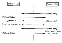
Device (B) rejects the data re-transmitted, and guits data transfer.
