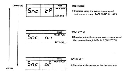
When the TR-626 is syncing to external devices, EXT SYNC will appear in the display. When you make the Display show tempo, the following sync mode is also displayed.
