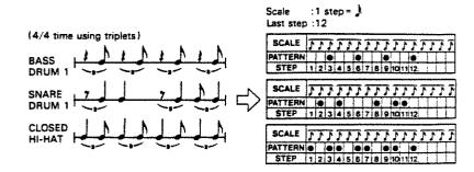
In a scale of thirty—two notes per step. 8 steps make a beat. Therefore, no more than two beats can be make with 16 steps. As a result of this, when a 4/4 time rhythm pattern is to be made, as in the figure, two patterns are used for writing it and then a single rhythm pattern is made by chaining them together. (See p.47.)
