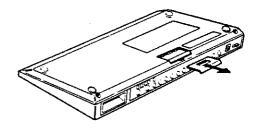
(3) Remove the batteries from the battery box, and replace them with new ones, are to match their polarities correctly (+ to + and - to -).
