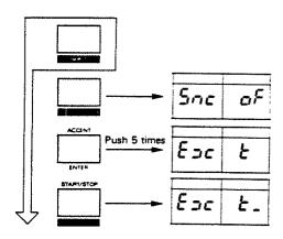
Step 4 When the transmission and the reception of data is being carried out correctly, the receiver TR-626 will display the following:
