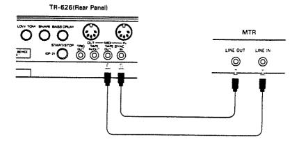
A pilot tone is constantly output through the TR-626's Tape SYNC Out Jack while it is stopped. Set the MTR recording level of the signal so that it is maintained between - 10 to -3 VU.
