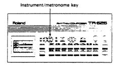
Pushing the Instrument / Metronome Key again will make the metronome stop.
