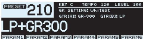
This screen shows the tempo, patch level, GK Setting, and COSM instruments.
