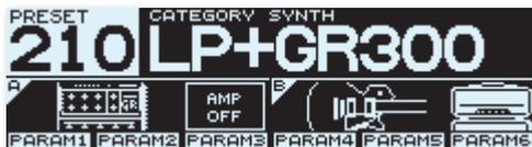
This Play screen variation shows icons that represent the COSM instruments and amps that are used in the patch.
