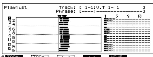
[F5 (WAVE)]: This displays the audio waveform for the corresponding track as selected using the [▲] and [▼] cursors. Press [F5 (WAVE)] once to display the waveform. Press [F5 (WAVE)] again to remove the waveform. (Make sure that the track you have selected contains audio.)
