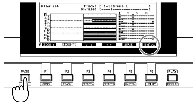
3. The mastering tracks can be turned off, or set to record or play back. [F6] toggles between these settings. The indicator above [F6] shows the setting that will be selected when you next press [F6], as indicated by an arrow. The current status of the mastering tracks can be viewed in the level meter in the display. For this example, press [F6] until “M→Off” appears above [F6]. Press [F6] once more to select this setting.
