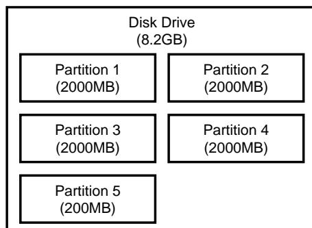
Each partition on the VS-1680's drive is treated as an independent drive, and is given its own partition number (0-7). When a single hard drive has multiple partitions, you can specify which partition of which drive will be used ("Drive Select," p. 222). The drive partition currently used is referred to as the "current drive."
