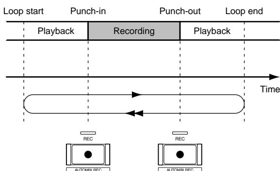
Before you begin recording, specify the begin and end times for the loop. There are three ways to specify the loop times. Use the method appropriate to your situation.
