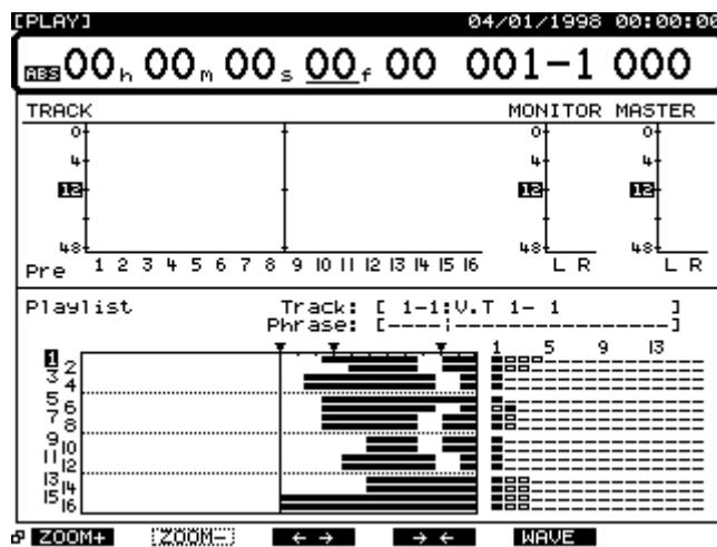
This display is separated into three different areas. You can use [▲], [▼], [◀], and [▶] as well as the Time / Value dial to change settings in each area. The currently active area is outlined with a bold line. Press [SHIFT] and [▲] or [▼] to change the currently active area.
