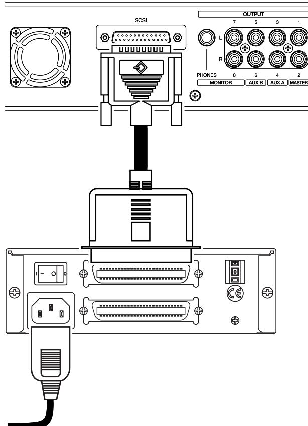
\* Once the connections have been completed, turn on the power to your various devices in the order specified. You can cause malfunction and/or damage to your speakers and other devices if you turn on devices in the wrong order.
