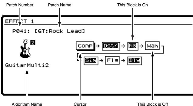
2. Press [ $\blacktriangleleft$ ] and [ $\triangleright$ ] to move the cursor in the screen. When you select a multi-effect patch (e.g., Guitar Multi 2), use the TIME/VALUE dial to turn each effect within that patch on or off. In the display, effect blocks that are currently activated and on are highlighted. Move the cursor to the highlighted effect block whose settings you wish to change.
