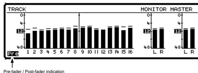
You can switch between Pre-fader and Post-fader by turning the TIME/VALUE dial or pressing [PAGE] until PRE or POST appears above [F4], and by then pressing [F4].
