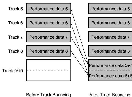
For this example, Tracks 5-8 are called the “source tracks.” Tracks 9/10 are called the “destination tracks.”
