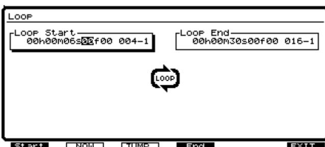
2. The loop start and loop end values appear in the display. Use [**<▶**] and [**▶**] to move the cursor to the value you want to adjust. If no value is stored, “—h—m—s—” appears in the display.
