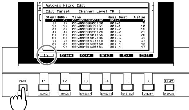
6. Make sure that the cursor is located at "Edit Target," and use the TIME/VALUE dial to select the Automix data that you wish to erase.
