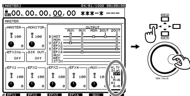
4. Select the mastering V-Tracks. Use [▲] or [▼] to move the cursor to “L:” or “R:,” and turn the TIME/VALUE dial to select the desired V-Track.
