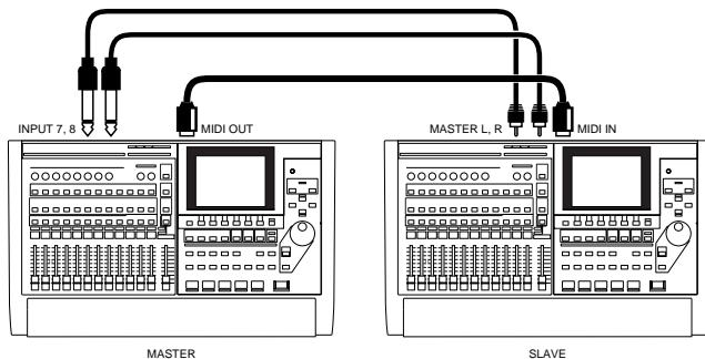
\* In this example, you can use the master's Stereo In function for the mix balance between the master and slave VS recorders (p. 185). First adjust the individual track balances on both machines. Of course, you can also send the output of both recorders to an external mixer.
