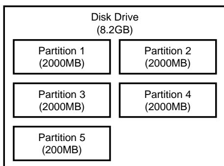
Each partition on the VS-1680’s disk drive is treated as an independent drive, and automatically given a partition number (0–7). When a single hard disk has multiple partitions, you can specify which partition drive will be used (“Drive Select,” p. 222). This selected disk drive partition used is referred to as the “current drive.”
