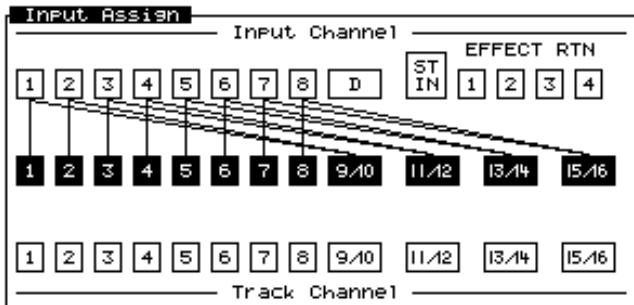
Using the STATUS and SELECT buttons, it is possible to set up almost any type of routing. To determine the source(s) assigned to a track for recording, use the following procedure.
