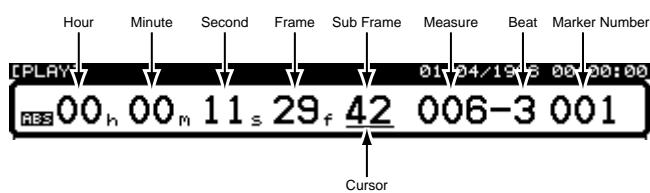
Turn the TIME/VALUE dial to change the playback time according to the position of the cursor. For example, if the cursor is positioned under the Minutes indicator, each click of the TIME/VALUE dial changes the timeline position by one-minute increments. If the cursor is moved to the subframe location, turning the dial moves the timeline position in increments of 1/10th of a frame. To move the timeline in 1/100th frame increments, hold [SHIFT] and turn the TIME/VALUE dial.
