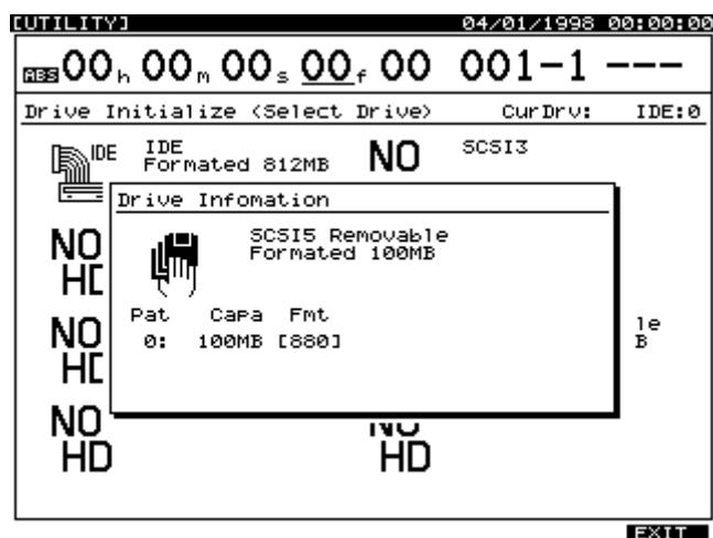
7. When the settings are made, press [F4 (Exec)]. “Initialize \*\*\* OK ?” appears in the display. “\*\*\*” refers to the selected drive’s SCSI number. For example, “SCSI5” indicates an external drive which is set to SCSI ID #5.
