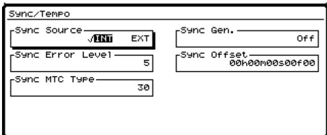
6. Use [▲], [▼], [◀], and [▶] to move the cursor to "Sync Gen.," and turn the TIME/VALUE dial to change the setting to "Off."
