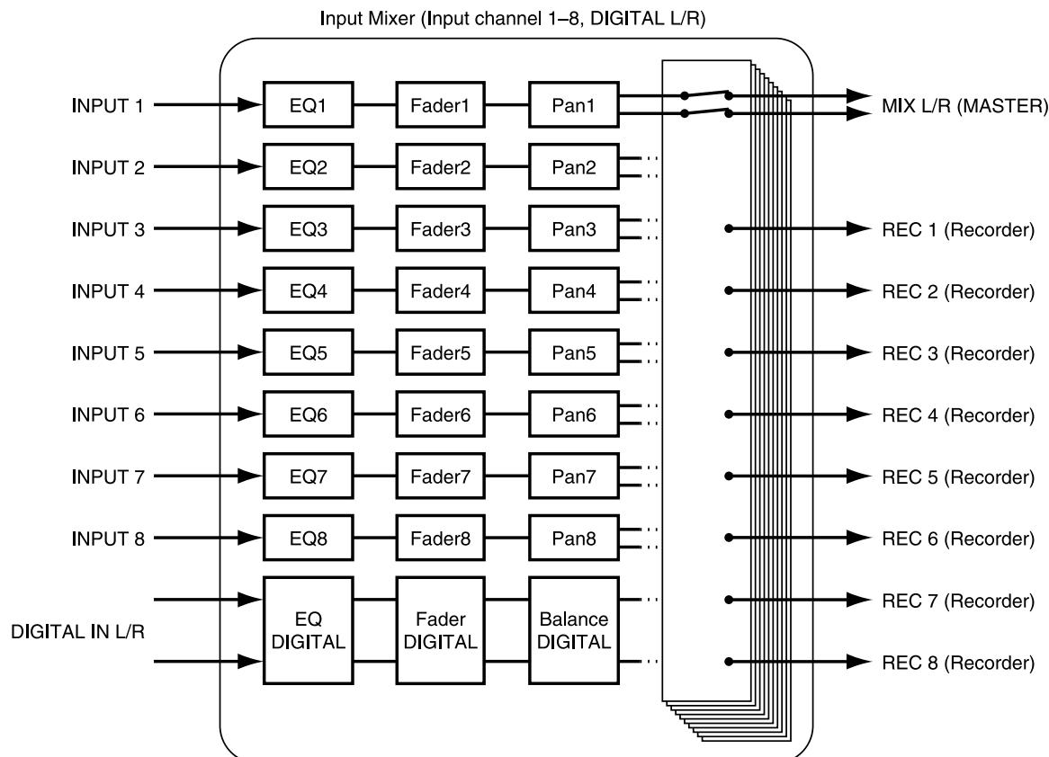
The output of each input channel is assigned to the track on which it is to be recorded. Channels not assigned to tracks are output directly from the MASTER jacks. Also, signals assigned to tracks when the tracks are not in Record Standby (STATUS indicator blinking red) are also output from the MASTER jacks. At this time, the following signals are assigned to the channel faders.
