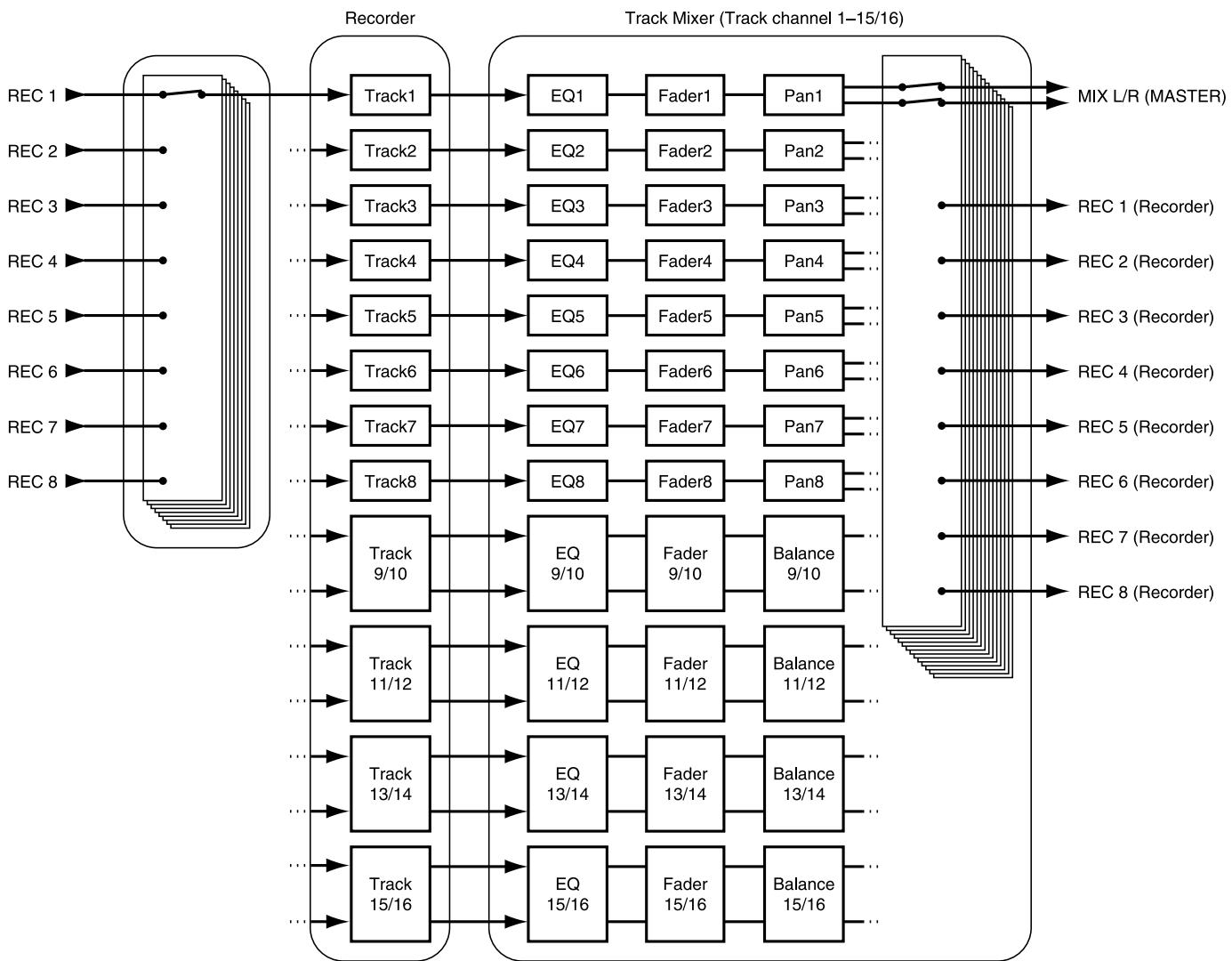
All of the tracks are output from the MASTER jacks. Additionally, tracks can also be routed back to the RECORDING bus for overdubbing, or re-recording. The channel faders 1–15/16 correspond respectively to Tracks 1–15/16
