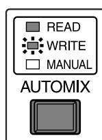
To begin using Automix, press [AUTOMIX]. The button indicator lights, indicating that Automix mode is on.
