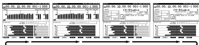
1. The initial screen shows level meters, the Playlist, and the V-Track Status grid. Hold [SHIFT] and press [PLAY (DISPLAY)] to switch to the next Playlist display.
