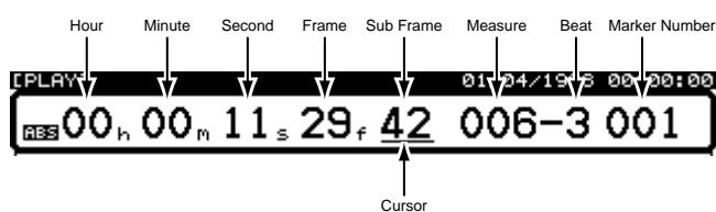
There are 100 Sub Frames in each frame. With the cursor at this position, each click of the TIME/VALUE dial advances the play position by 11 hundredths (11/100th) of a frame. Hold [SHIFT] and slowly turn the TIME/VALUE dial. Now each click moves the edit line by exactly one hundredth of a frame. One hundredth (1/100th) of a frame is equivalent to one three thousandths (1/3,000th) of a second.
