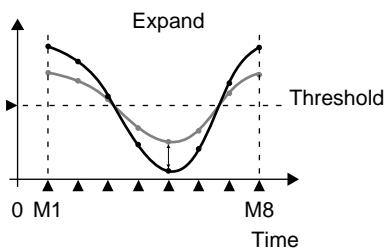
11. To execute the Shift/Expand operation, press [F4 (Exec)]. If you press [F6 (EXIT)], you will return to Step 7 without executing the Shift/Expand operation.
