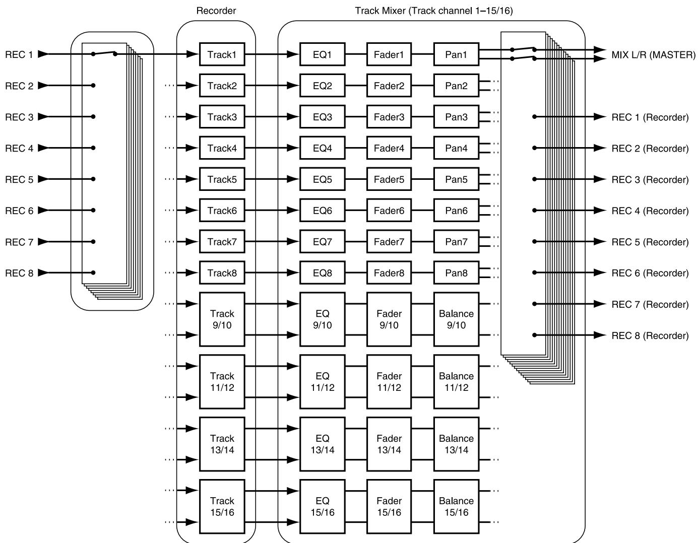
Tracks are normally output from the MASTER jacks. Tracks can also be routed back to the RECORDING bus for track bouncing or re-recording, or to individual outputs for transferring to other multitrack recorders using the Direct Out function.
