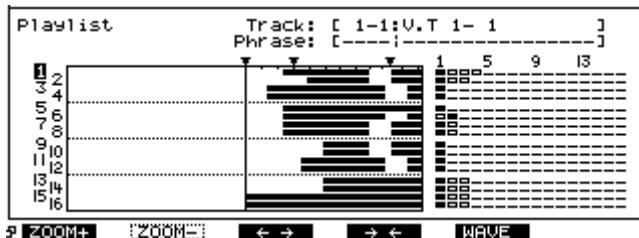
[F3 (<->)]: This stretches the timeline in four stages. When a waveform is displayed, this laterally stretches out the waveform.
