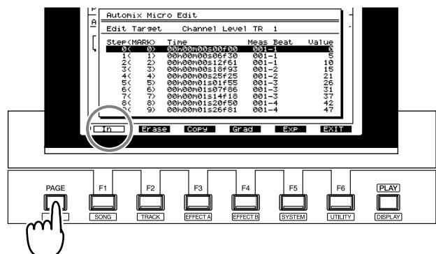
6. Make sure that the cursor is located at "Edit Target," and use the TIME/VALUE dial to select the type of Automix
