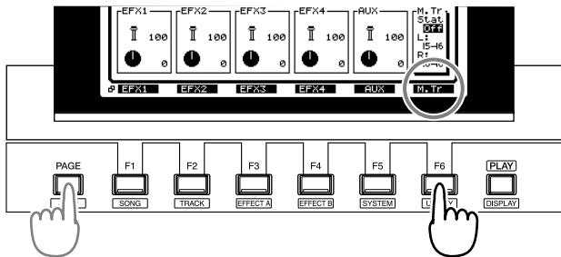
3. Select the status of the mastering tracks. Make sure that the cursor is located at “Stat,” and then turn the TIME/VALUE dial.
