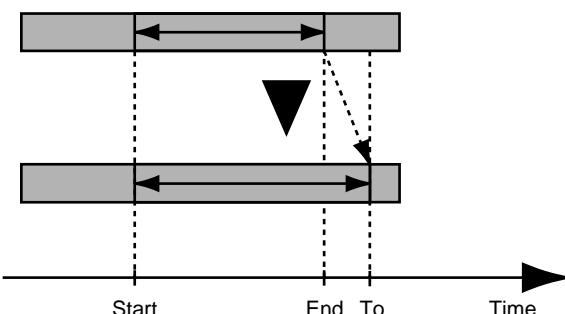
\* *Track Compression/Expansion creates new performance data with a different playback time. For this reason, it cannot be executed if there is not sufficient space on the current drive.*
