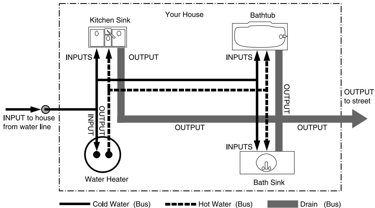
If we think of the VS-1680 as the house, the water being supplied from the water company corresponds to inputs such as mic or guitar. Some of these inputs are sent to recording tracks and are recorded. Other portions are sent to the effects, and reverb or chorus are applied before they are output.
