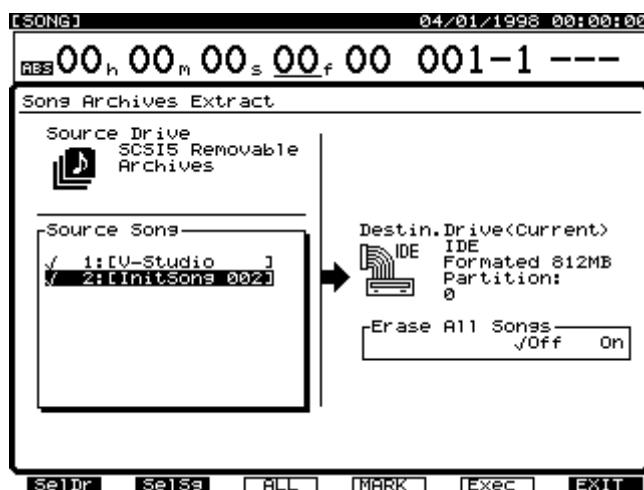
6. If several external drives are connected to the VS-1680, press [F5 (SelDr)] to view a list of drives. Use CURSORS to select the drive that contains the Song Archive disk, and press [F1 (Back)].
