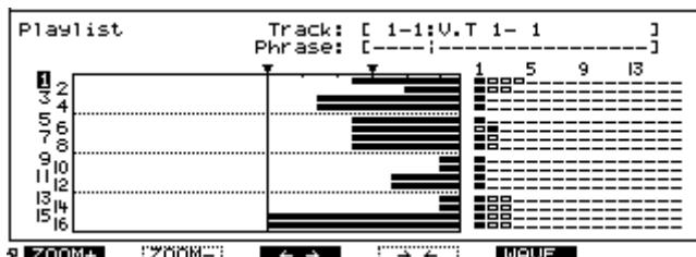
[F4 (-><-)]: This shrinks the timeline in four stages. If a waveform is displayed, this will squeeze the waveform.
