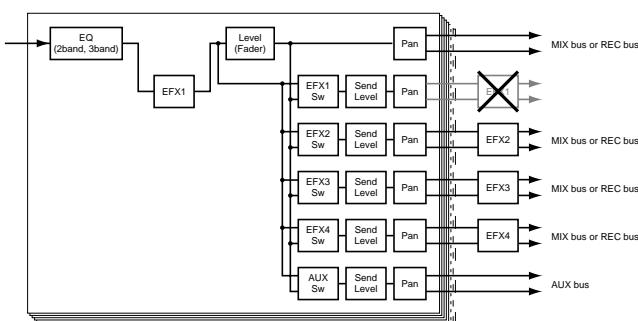
\* Depending on the effects used, when mixing with different effects inserted into each channel, or mixing some channels
