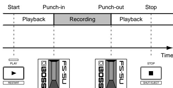
Connect the optional foot switch to the VS-1680's FOOT SWITCH jack.
