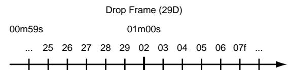
Non-drop is generally used for most video and audio productions, since formats with continuous frames are easier to deal with. In contrast, in situations such as live broadcasts, where the time code clock must match actual clock time, drop frame is used.
