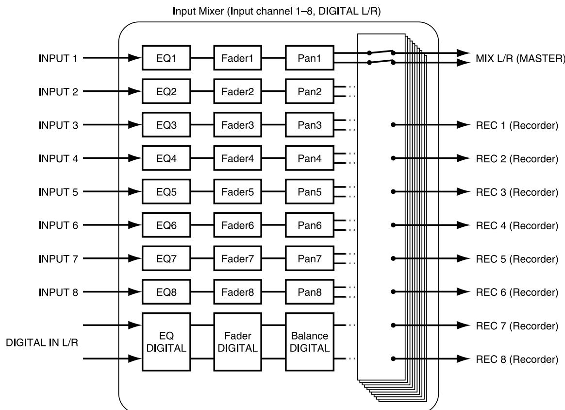
The output of each channel of the Input Mixer can be assigned to tracks to be recorded. Channels not being recorded can be assigned to the MIX bus for output from the MASTER jacks. When an input is assigned to a track for recording, it can also be monitored from the MASTER jacks when the track's STATUS button is orange or blinking red.
