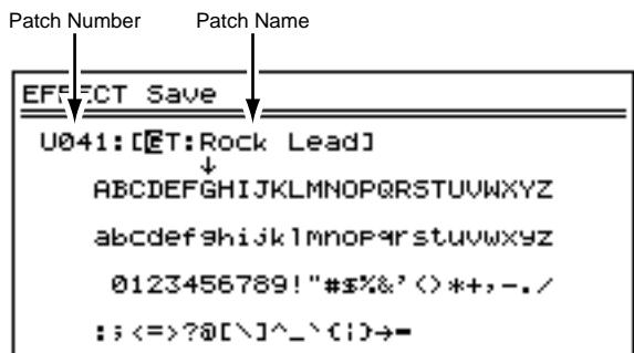
3. Use [◀] and [▶], and the TIME/VALUE dial to create the name of the user patch. The function buttons work as shown:
