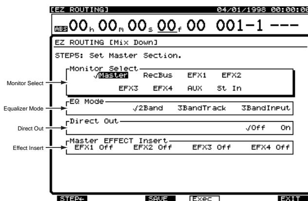
13. Press [F4 (Exec)]. "EZ ROUTING Step Edit is finished!!" appears in the display.
