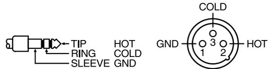
Some audio devices employ the opposite HOT (TIP) and COLD (RING) wiring. Using such equipment as is may result in poor sound placement, loss of correct left-right balance, and loss of separation between left and right channels when using stereo inputs. In such cases, you need to switch the phase of each channel.
