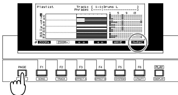
3. Press [F6] until "M→Ply" appears above [F6]. Press [F6] once more to select this setting. The current status of the mastering tracks is shown in the display.
