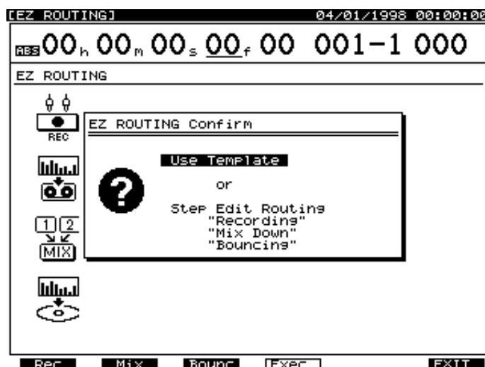
4. Press [◀] and [▶] to move the cursor to “Use Template” and press [F4 (Exec)] once more. “Apply this ROUTING ?” appears in the display.
