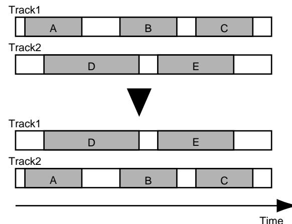
1. Select the V-Track containing the source playback audio to be exchanged.
