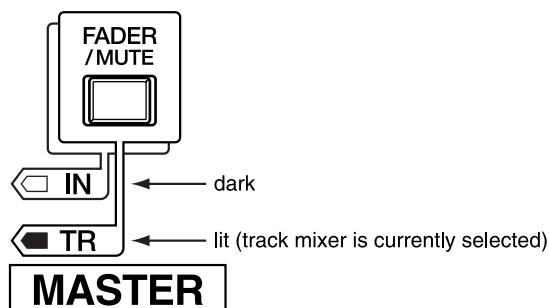
When "TR" is lit, the physical faders are used to control the Track Mixer Channels 1-16.
