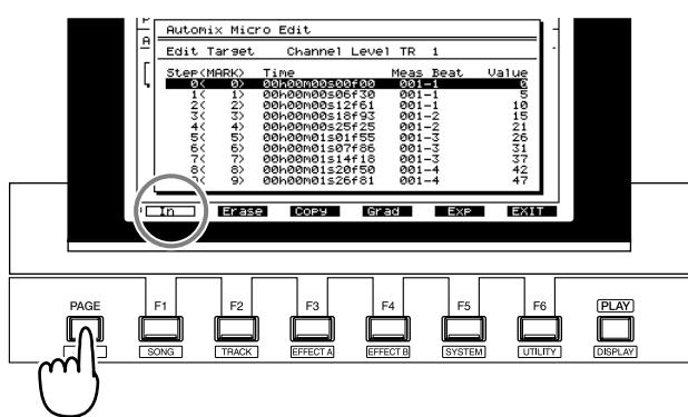
6. Make sure that the cursor is located at “Edit Target,” and use the TIME/VALUE dial to select the type of Automix data that you wish to edit.
