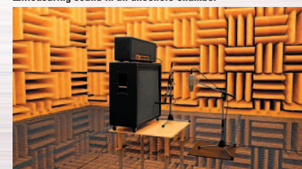
■ Measuring sound in an anechoic chamber
