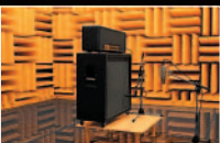
●Measuring sound in an anechoic chamber
