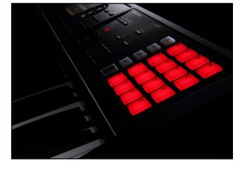
level. In addition to sample triggering, the pads can be used for numerous functions such as muting parts, entering numeric values in the display, and more.
