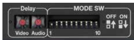
Delay Dials (VC-1-DL only) and DIP switches on side panel
