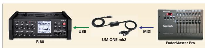
When space allows, buttons and faders can streamline your field recording workflow. With the Roland R-88, you can easily expand your work surface to include a MIDI fader controller. Connect your device to the R-88 using a Roland UM-ONE mk2 USB MIDI interface and mixing becomes a breeze. A video and setup guide are available demonstrating the use of the JL Cooper FaderMaster Professional, as one example.
