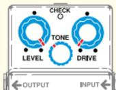
Set DRIVE at a lower level and turn LEVEL all the way up. With this setting, the SD-1 functions as a gain booster, augmenting amp distortion and providing deeper, thicker sounds.
