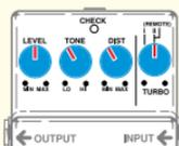
Turbo Mode II gives you a full mid-range sound. Set DIST at a moderate level to obtain a rough, street-level sound. This setting is ideal for hard rock chord work.
