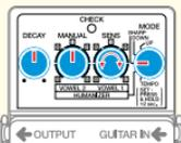
To get more of a synth-type filter sound, adjust the SENS knob to suit your picking strength, and turn the MODE knob to SHARP.
