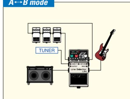
This setup is for switching between an effects loop and tuner. Switch to mode B during live performance for silent tuning.
