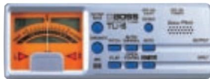
The TU-15 is BOSS' ultimate tuner, offering renowned needle-point accuracy, a backlit display, flat tuning, and a host of "world's first" features not found in any other tuner. Especially noteworthy is the new "Accu-Pitch" function, which sounds a note when the correct tuning is reached.
