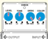
Turn the COLOR control all the way to the OD side. With this setting, the OS-2 functions strictly as an overdrive effect. Turn DRIVE all the way up to MAX to get hard distortion. This is a perfect sound for Humbucking pickups.
