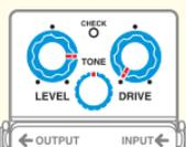
This setting boosts amp gain, resulting in powerful distortion. The key is to limit the DRIVE knob to the 9 o'clock position and, for the ultimate in distortion, to push the LEVEL control to the max.
